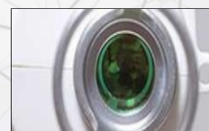
The Spot Size diameter is (in microscope) <70um, which has penetrate depth 2mm.
